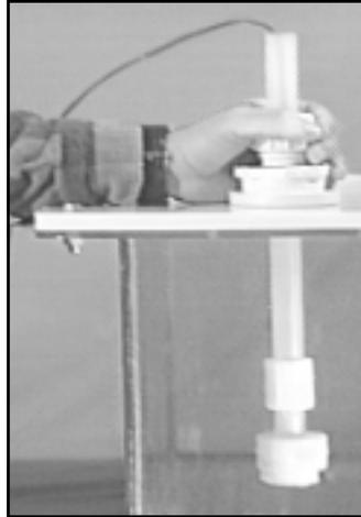
1. Loosen the mounting bracket compression nut.
